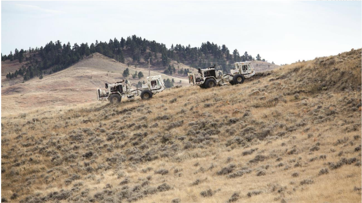
Figure 2. Vibroseis trucks are used to conduct 3-D VSP surveys in the Bell Creek Field.
