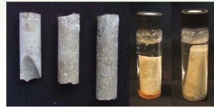
al Sample After exposure After exposure After exposure (CO2) (CO2+H2S) (CO2) (CO2+H2S)
