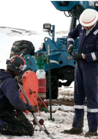
Postinjection monitoring activities continued for 90 days. Two of the activities were gas sampling and crosswell seismic tomography to track CO 2 movement deep underground.
