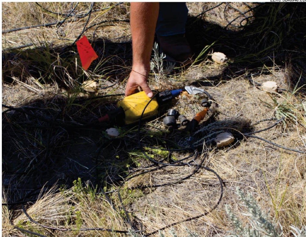
Figure 13. GSR (geospace seismic recorder) recording unit with geophones planted in a 2-ft circle.
