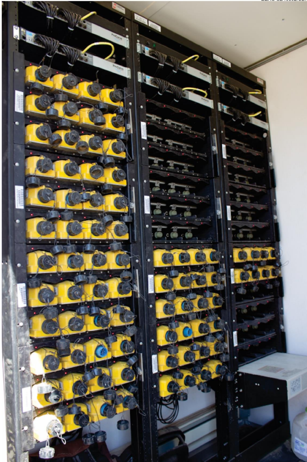
Figure 14. Nodal recording units in a rack used for operational checks, programming, and data collection.
