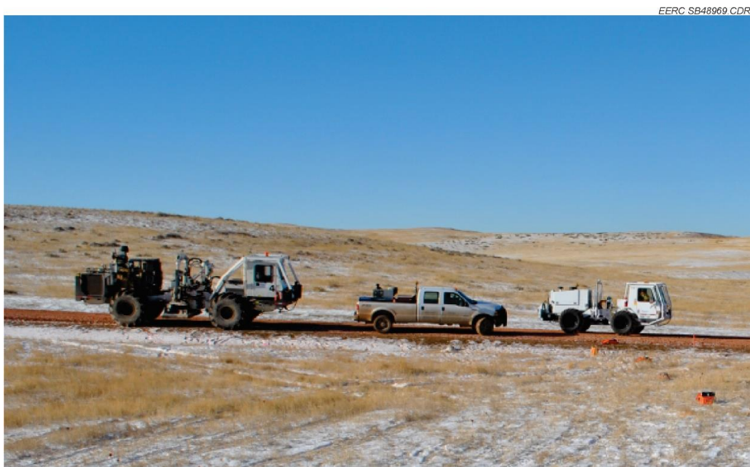
Figure 7. An I/O AHV-3 heavy vibrator (left) and an IVI Minivib Vibrator on a field road at Bell Creek during the December 2011 source testing.
