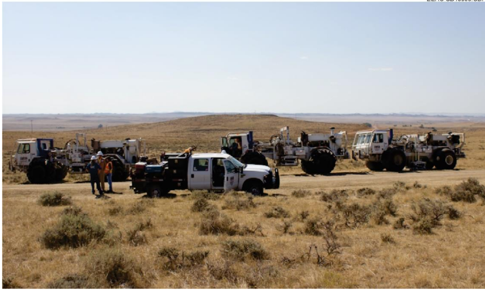
Figure 15. Vibrator crew during Bell Creek survey. Two units shook together at each shotpoint. The third unit is a spare.
