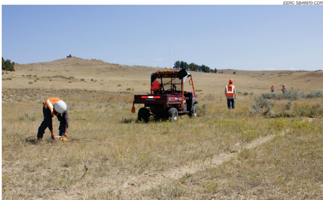
Figure 12. Seismic crew members laying out receiver stations.
