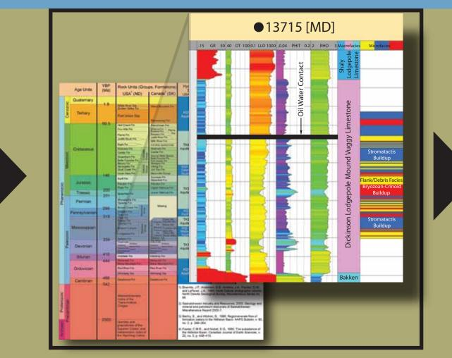
Core data, core images, and wireline logs were used to determine macrofacies and microfacies logs, formation tops, and the oil—water contact (OWC).
