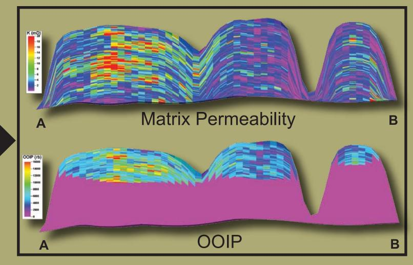
Cross-sectional output for reservoir logistics and dynamic model. An indicator volume was produced representing volume of oil (ind=1) and volume of water (ind=0). This volume was then multiplied by effective pore volume to acquire OOIP.
