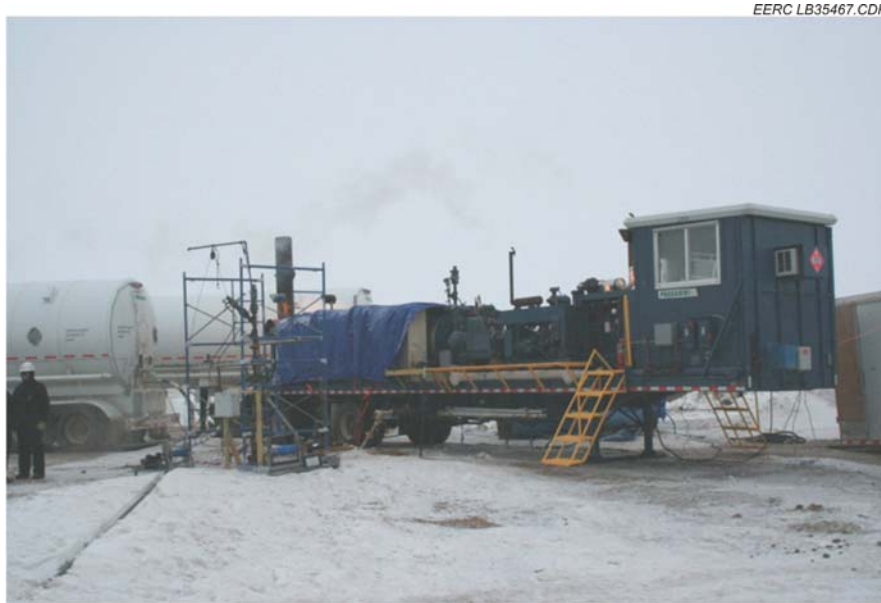
Figure 4. Site photo of pump skid and CO 2 storage tank.
