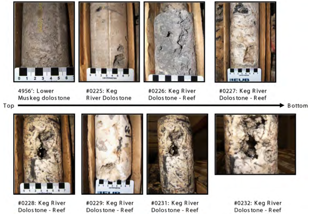
Figure 2. Core samples illustrating the heterogeneity of the Keg River Pinnacles that are being utilized in the Zama Project.
