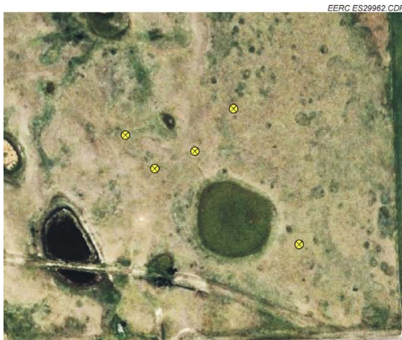
Figure 1. Wells configuration for the lignite test in Burke County, North Dakota.
