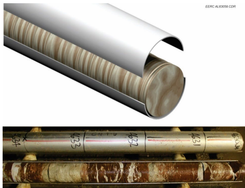
Figure 6. Top: Half-moon liner system that allows viewing of the core at the rig site (Reservoir Group, 2022). Bottom: Field photo of core collected from a stratigraphic test well using the half-moon liner system.
