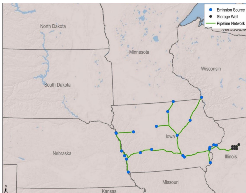
Figure 11. A SimCCS Gateway hub network layout targeting 90% of the total network CO 2 source emissions (43 million metric tons annually).
