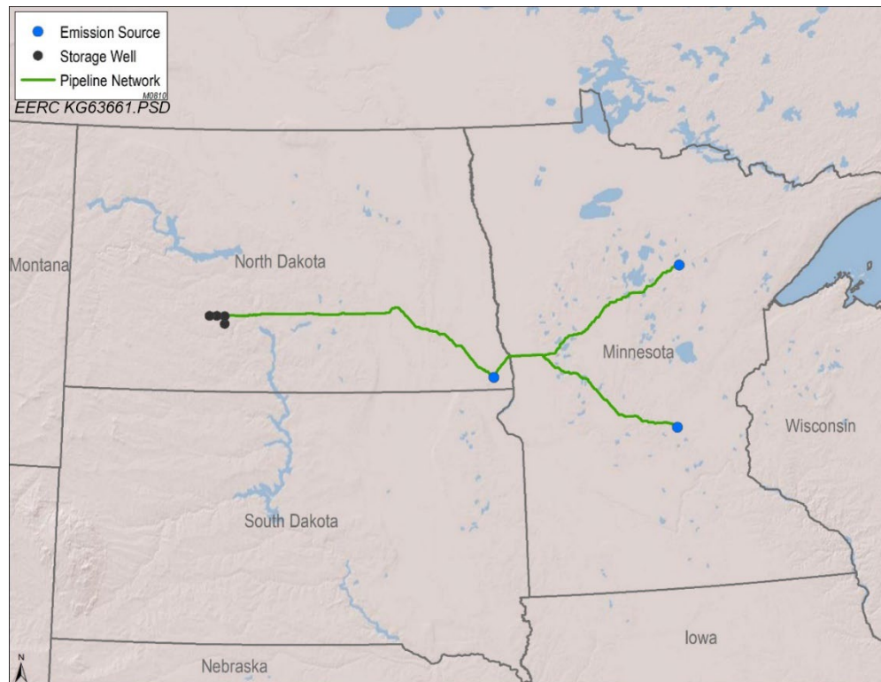
Figure 6. An optimized network layout targeting 33% of the total network CO 2 source emissions (16.8 million metric tons annually).
