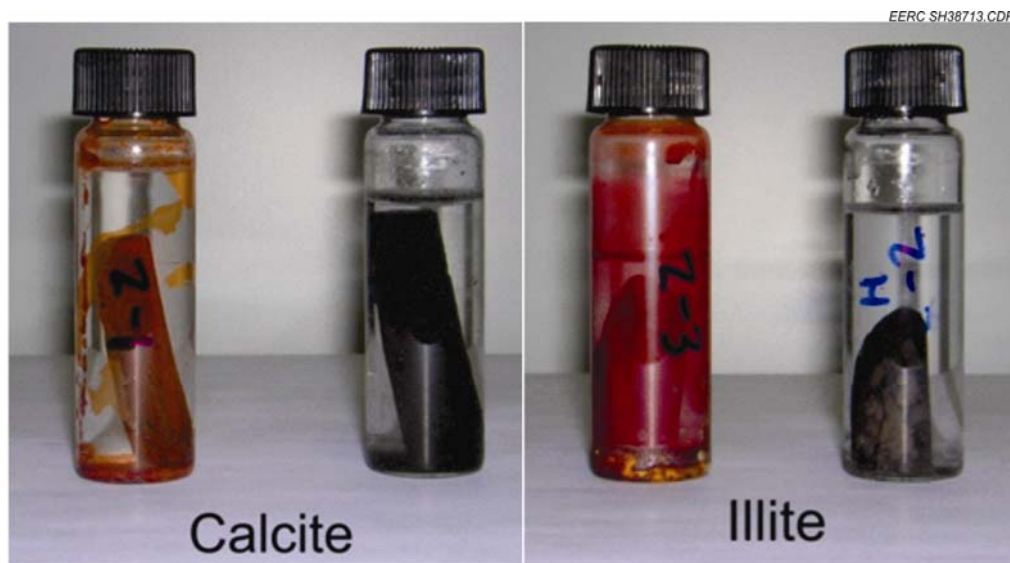
Figure 4 Changes in calcite and illite minerals when exposed to pure CO 2 (left vial in each photo) and acid gas (right vial in each photo). Discussions of the mineralogical reactions that occur under pure CO 2 and with acid gas are in Paper 1117.00.
