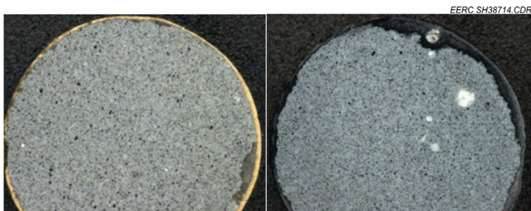
Figure 3 Wellbore cement exposed to pure CO 2 (left) and to acid gas (right) for 28 days.
