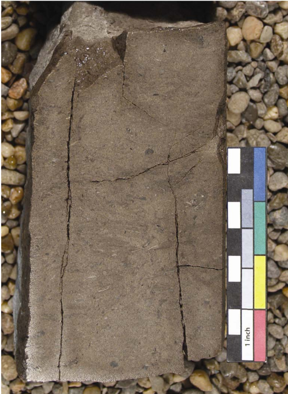
Figure 11. An example of a core sample from the E. Goetz No. 1 well. Note the vertical fractures, the analysis of which from this core and many others from the study area allowed for prediction of fracture distribution within the Mission Canyon Formation in the Northwest McGregor Field.
