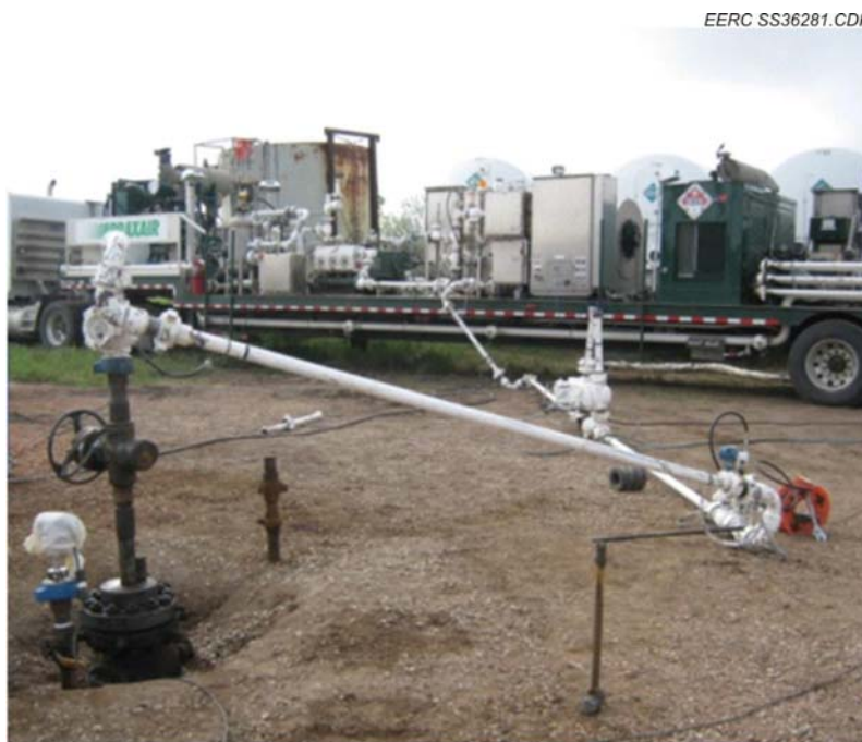
Figure 21. Pumping unit and pipe and valve system used to inject CO 2 into the E. Goetz No. 1 well.
