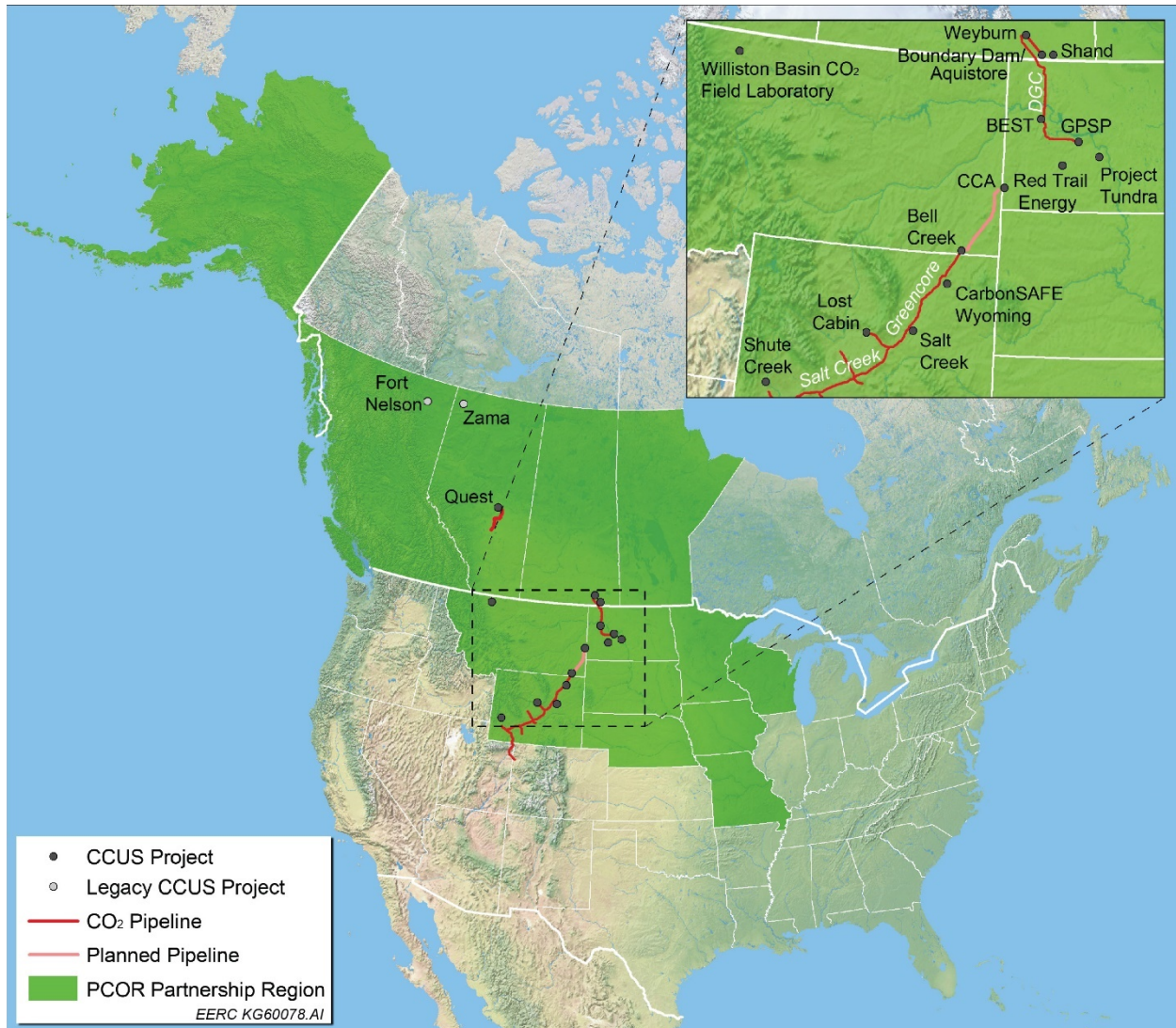
Figure 1. Proposed PCOR Partnership region showing focus areas, pipelines, and CCUS projects. GPSP stands for Great Plains Synfuels Plant. BEST stands for Brine Extraction and Storage Test. CCA stands for Cedar Creek Anticline. DGC stands for Dakota Gasification Company.
