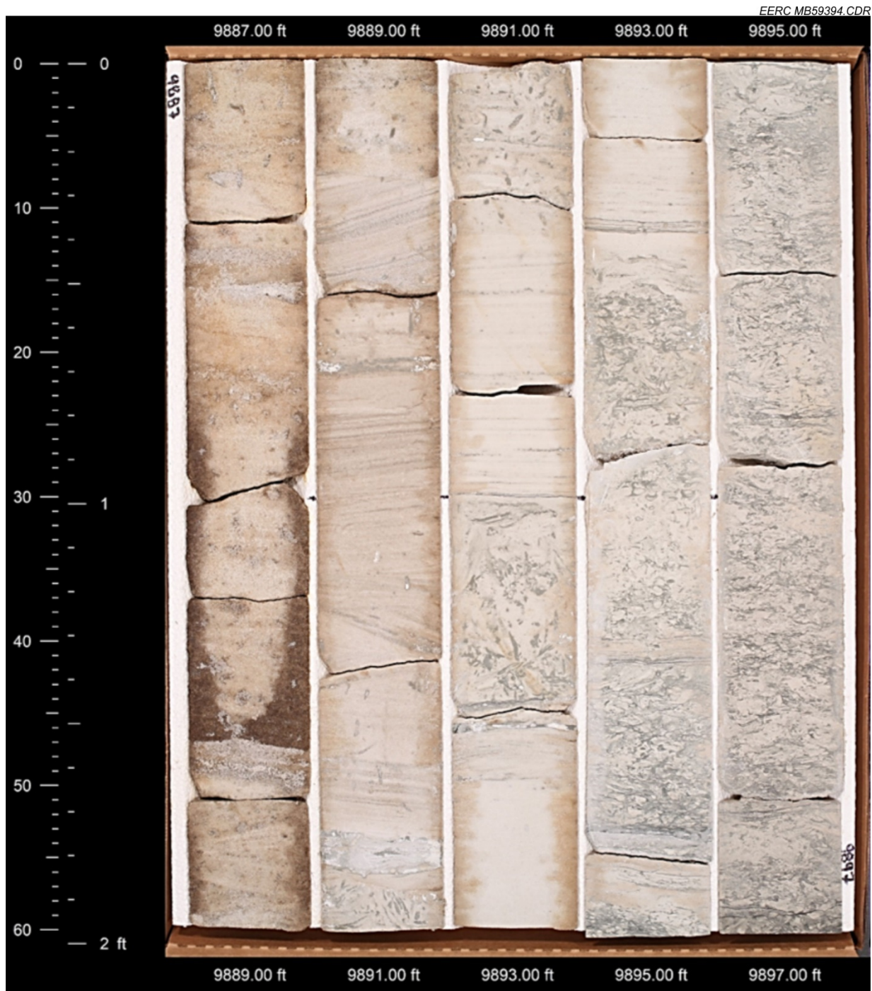
Figure 6. Core samples from the upper reservoir of the BCS, acquired in the J-LOC1 well (NDIC File No. 37380). The recorded depths of this interval are from 9887 ft (upper left) to 9897 ft (lower right), grading from an unstructured quartz sandstone at the top down through cross-bedded sandstone and then into a sandy mudstone with lenticular and wavy, fine-grained interbeds. This well was drilled with an oil-based mud, which is the cause of the dark brown staining from 9888 to 9889 ft.
