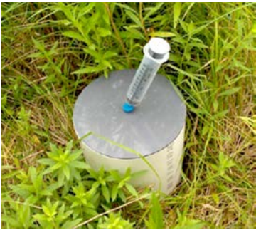
Gas exchange was sampled biweekly (right) from static chambers transecting uplands and wetlands under different land uses (bottom).
