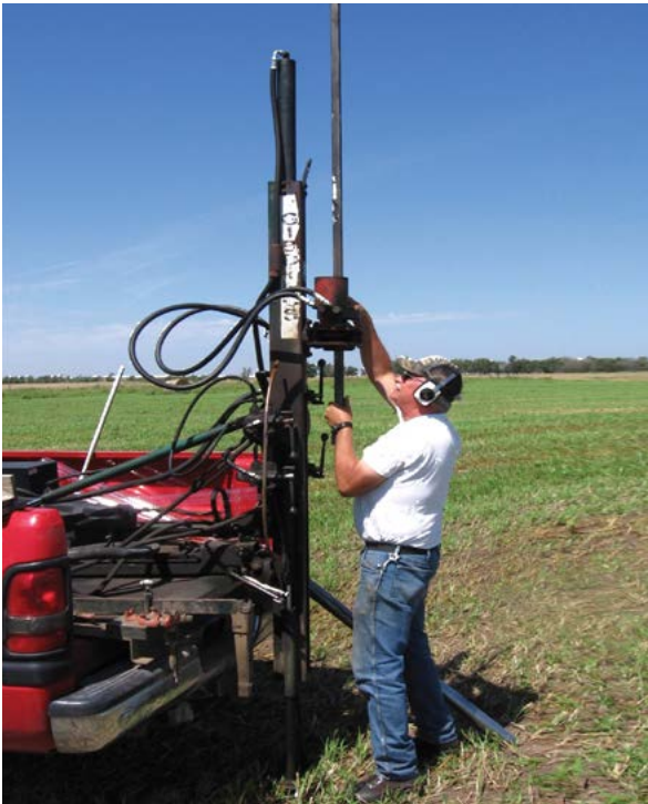
Soil-profile cores were extracted during the course of the study to measure changes in soil carbon at different depths.
