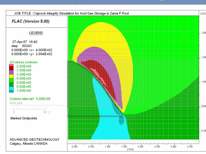
assess the magnitude of stresses developed in the reservoir and the caprock as a consequence of initial il production, subsequent waterflooding, and more recently acid gas injection we are using the leformations, induced normal and shear stresses, and to assess the propensity for fault re-activation of adjacent to the F pool pinnacle reef at a reservoir pressure of 28 MPa. Vertical exaggeration is 2:1.
