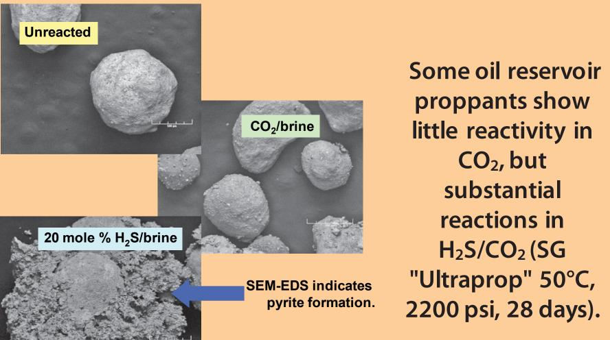
proppants show little reactivity in CO<sub>2</sub>, but substantial reactions in H<sub>2</sub>S/CO<sub>2</sub> (SG "Ultraprop" 50°C, 2200 psi, 28 days).
