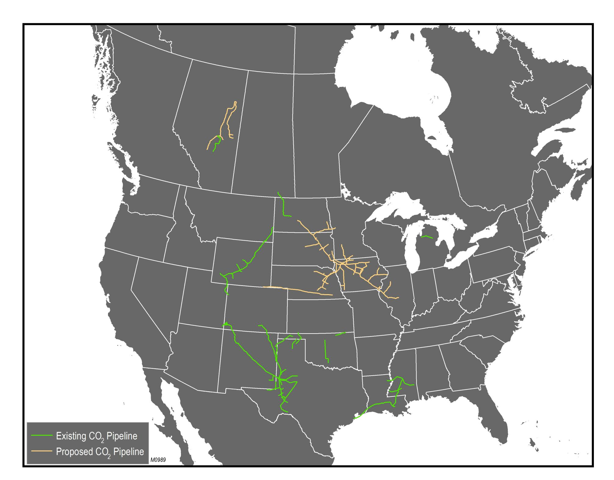
There is >9630 km (5985 mi) of CO<sub>2</sub> pipeline in North America, touting a maximum capacity >225 Mt/yr:
