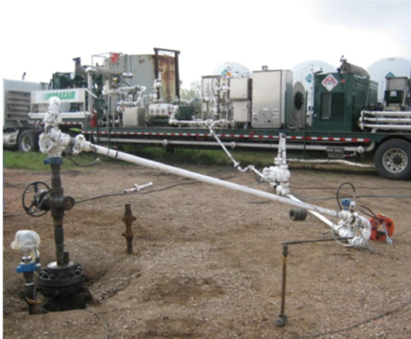
Figure 4-7. Pumping unit and pipe and valve system used to inject CO 2 into the E. Goetz #1 well.
