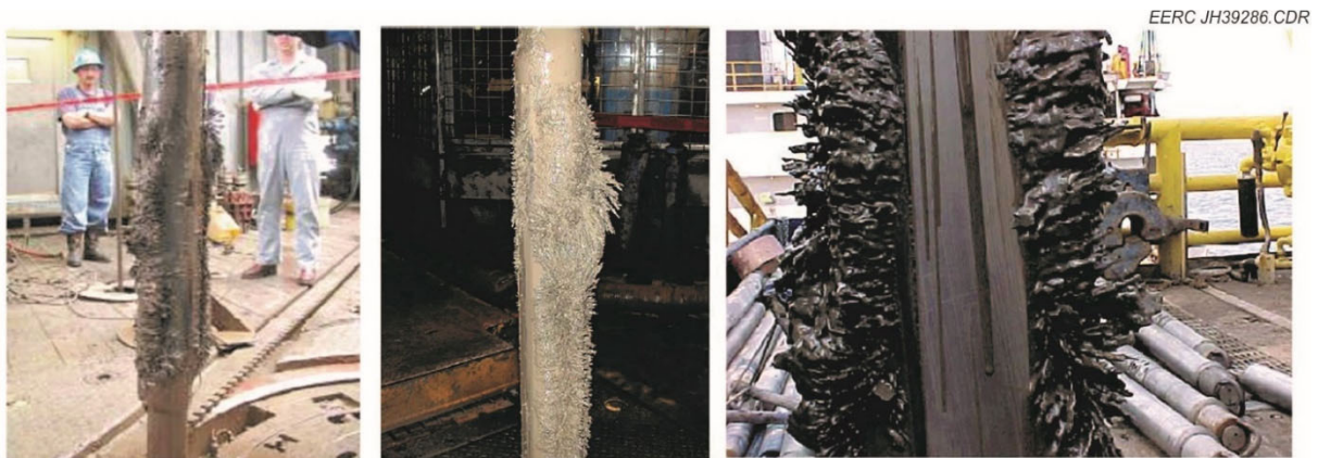
Figure 12. Multiple images illustrating magnetic debris buildup on the permanent magnets of an NMR tool after a logging run. Ditch magnets will reduce the amount of debris present in the borehole prior to logging and, therefore, reduce the metallic buildup, potentially improving measurement quality and reducing the time necessary to record measurements (Minh and others, 2005).
