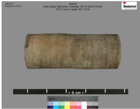
Figure 5: Full Diameter Core from 5012 m
