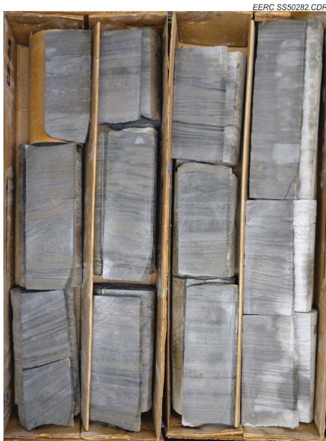
Figure 2. Example of slabbed core viewed and described prior to sampling.
