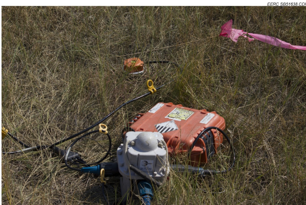
Figure 3. Nodal geophone assembly on station. From the top, a pin flag marking the surveyed receiver location, three-component geophone with leveling bubble, field battery, and Sercel Unite digital acquisition unit with GPS (global positioning system) antenna dome.
