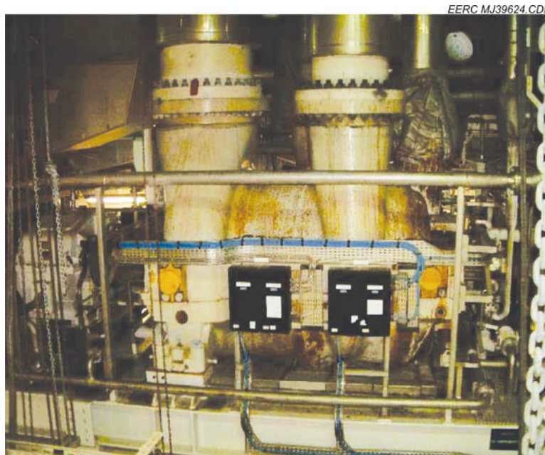
Figure 8. A two-stage in-line compressor (taken from Miller, 2009). This compressor, at the Sleipner project, compresses a million tonnes of CO 2 each year from 0.1 to 0.4 MPa (14.5 to 58 psi) in the first stage and 0.4 to 1.5 MPa (58 to 218 psi) in the second stage. An additional two stages produce a final pressure of 6.6 MPa (957 psi).
