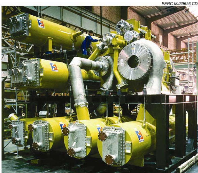
Figure 10. A ten-stage integrally geared centrifugal compressor (at Azot Nowomoskowsk in Moscow, Russia) shown with its intercoolers. It can compress 391 \text{ m}^3/\text{minute} (13,800 acfm) wet \text{CO}_2 from 0.1 to 20 MPa (15 to 2900 psi) (taken from Kisor, 2009).
