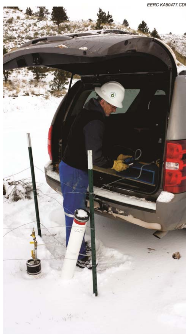
Figure 19. EERC field personnel monitor soil gas concentrations at a SGPS in the Bell Creek Field (March 2014).
