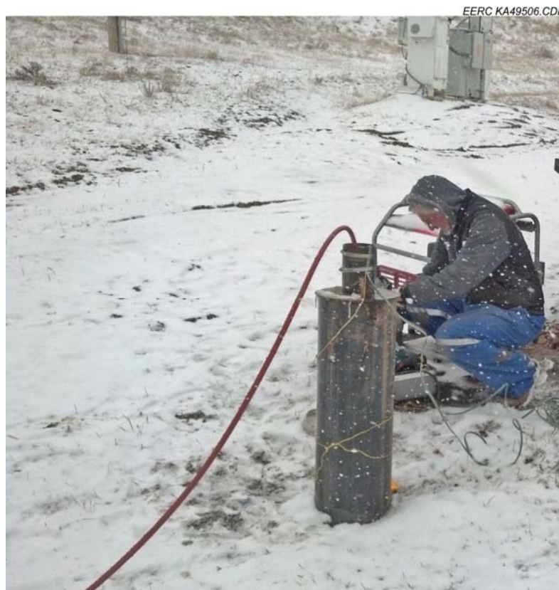
Figure 20. EERC field personnel record water table elevation data and purge a minimum of three well casing volumes during groundwater monitoring at the MW33-12 monitoring well (Fox Hills) (February 2014).
