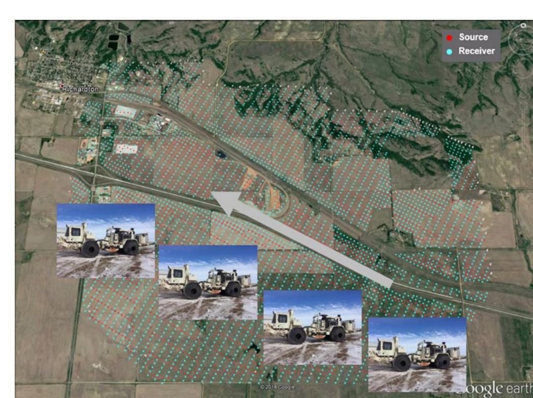
Location of seismic sensors deployed for a SASSA noise test within the same 8-square-mile area investigated with the 3D seismic survey conducted in 2019.
