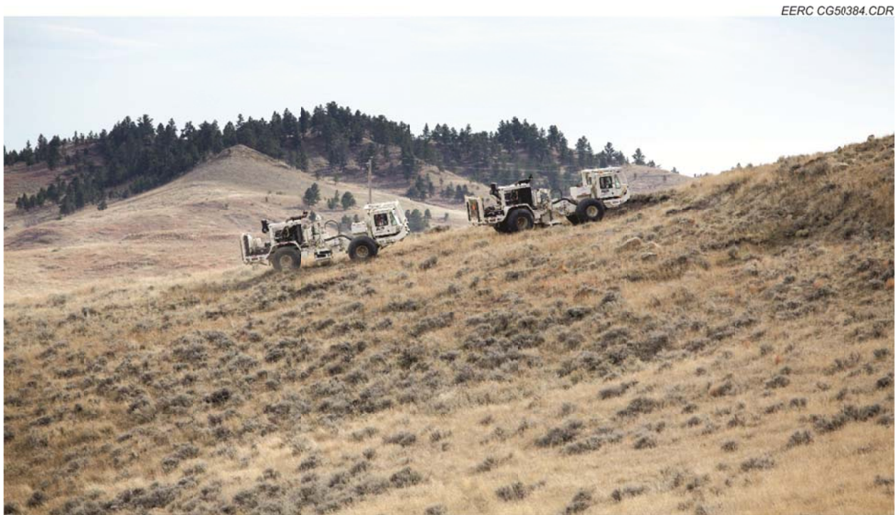
Figure 7. Vibroseis trucks are used to conduct 3-D VSP surveys in the Bell Creek Field.
