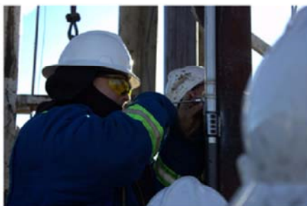
Promore engineer connecting a pressure/temperature gauge to the casing-conveyed PDM system on the rig floor.
