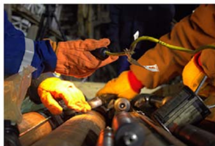
Schlumberger perforating specialists arm the casing-conveyed perforating charges on the PDM system.
