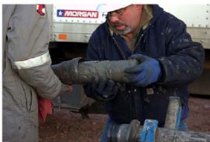
A Baker Inteq coring specialist removing a piece of full diameter core from the core barrel at the 0506 OW well site.
