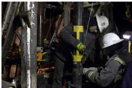
Promore, Qorex, and BMP engineers attaching a centralizer to the casing to protect capillary lines and the multiconductor cable which provides data transmission between the PDM equipment and the wellhead.
