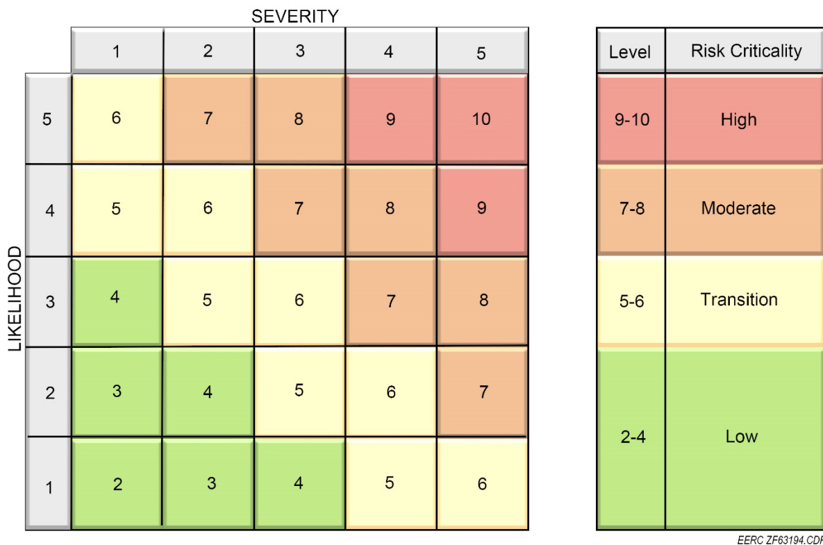
Figure 7-4. Example risk map and suggested actions using five-point risk likelihood and severity scales.
