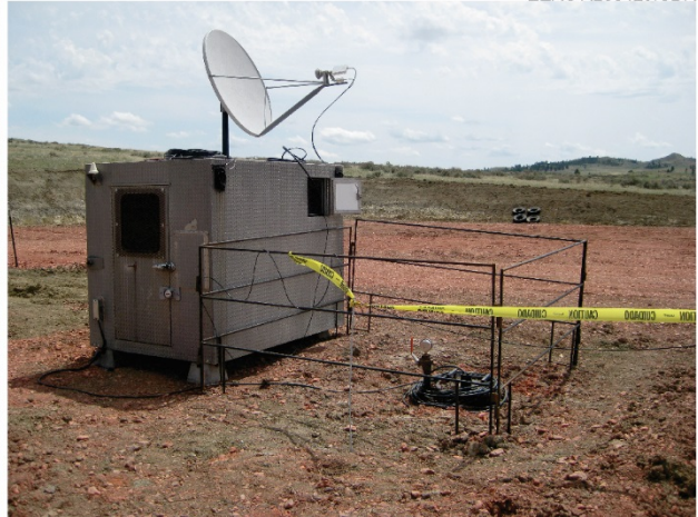
Figure A-8. Photos of the 04-03 OW wellhead showing the fiber optic cable running from the borehole array to the surface (left) and 04-03 OW recording shack (right). The satellite Internet dish allowing remote operation is mounted on top of the shack.
