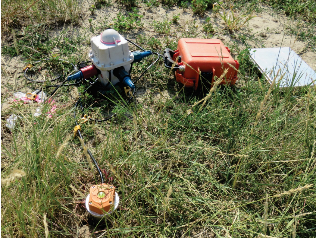
Figure 13. 2015 monitor and baseline extension survey receiver stations employed the DTCC (Dynamic Technology Canada Corporation) DT-Solo 3-component 10-Hz geophone, a Sercel UNITE data logger, and battery.
