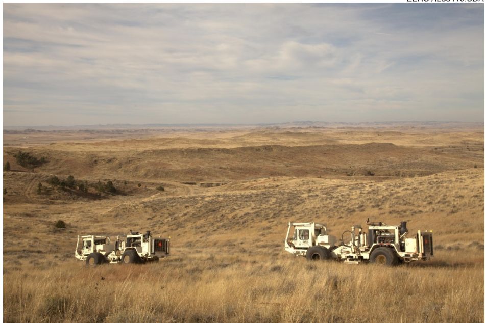
Figure 10. Two Vibroseis trucks moving between shot points during the 2014 monitor survey.
