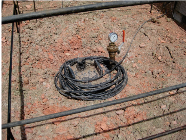
Figure A-8. Photos of the 04-03 OW wellhead showing the fiber optic cable running from the borehole array to the surface (left) and 04-03 OW recording shack (right). The satellite Internet dish allowing remote operation is mounted on top of the shack.
