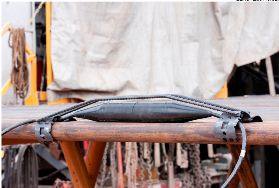
Figure A-5. Photo of the rebar cage and clamp used to secure and protect the sensor modules.
