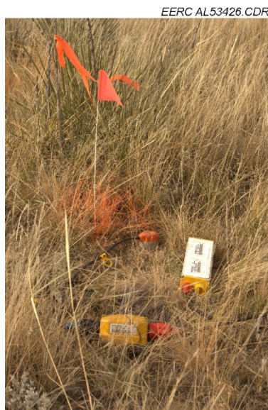
Figure 11. 2014 monitor survey receiver station with a single GS-1, 3-component 10-Hz geophone (center), Geospace GSX seismic recorder (bottom), and battery.
