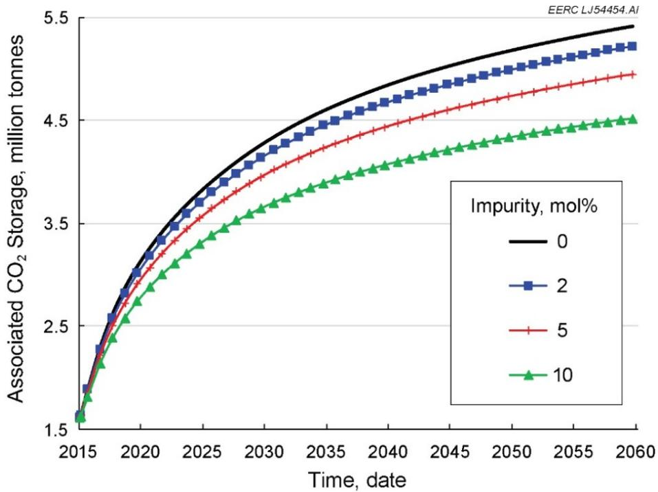
Figure 9-10. Associated CO<sub>2</sub> storage performance for recycled gas injection with varying impurity content.
