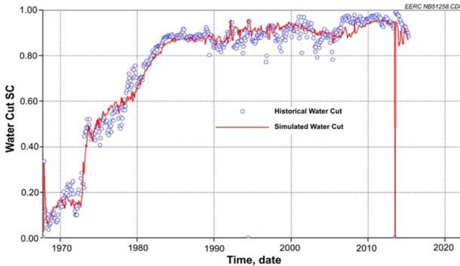
Figure 9-5. Water cut history match results for Phase Areas 1 and 2 of the Bell Creek oil field using the refined reservoir simulation model (Jin and others, 2016a).
