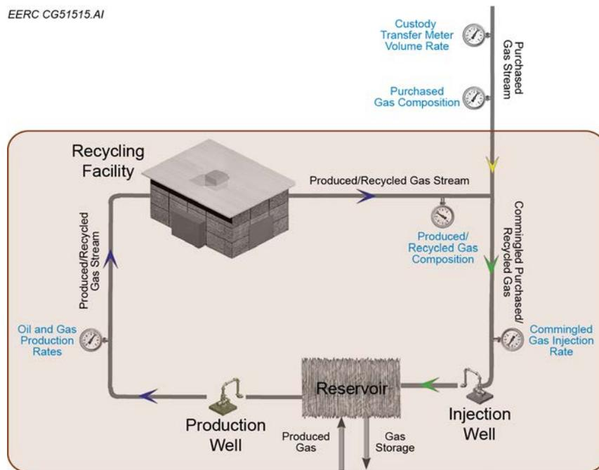
Figure 18. Simplified CO<sub>2</sub> EOR injection and recycling system.
