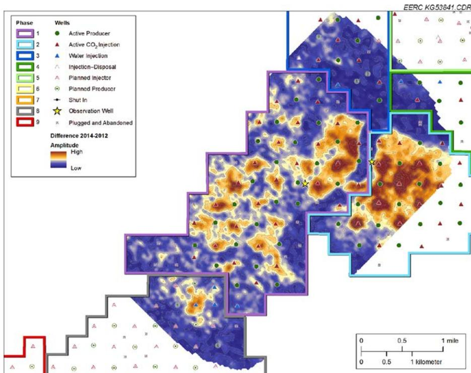
Figure 9-4. Time-lapse difference of 4-D seismic surveys conducted in Phase Areas 1 and 2 of the Bell Creek oil field in September 2012 and November 2014. (modified from Salako and others, 2017).
