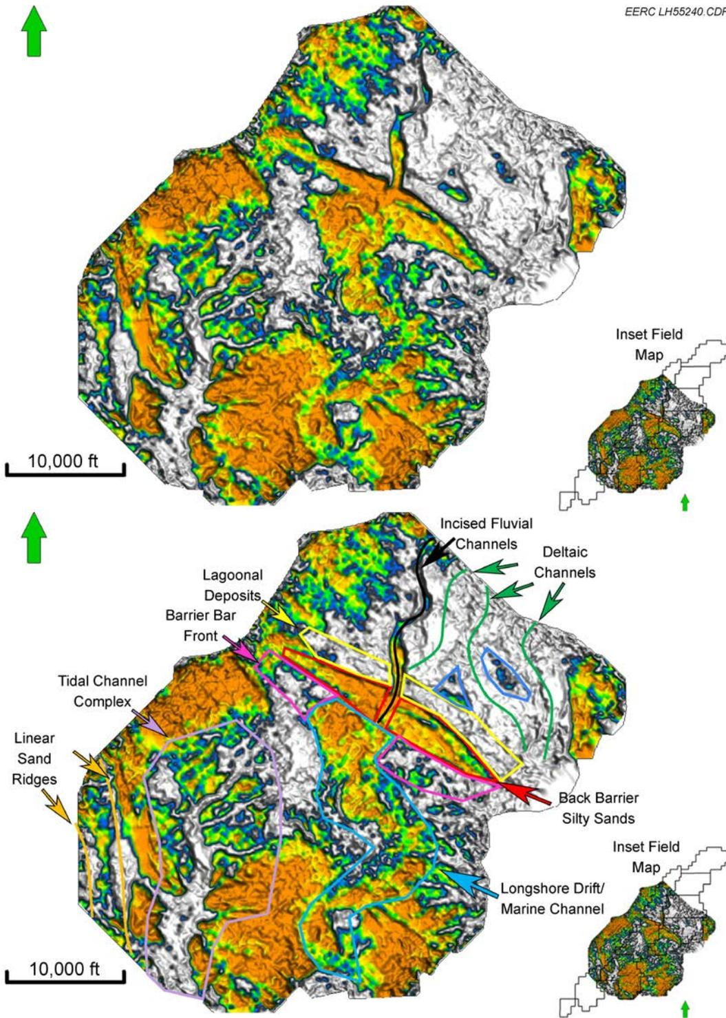
Figure 9. Amplitude summation map calculated over the Muddy Formation interval of the Bell Creek Field (top; adapted from Burnison and others, 2014) and an annotated version of the map identifying interpreted geobodies (bottom).
