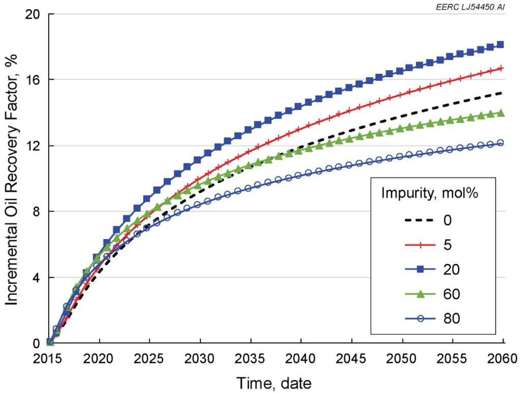
Figure 9-9. Comparison of oil recovery factor for WAG operations using recycled gas injection with varying impurity content.
