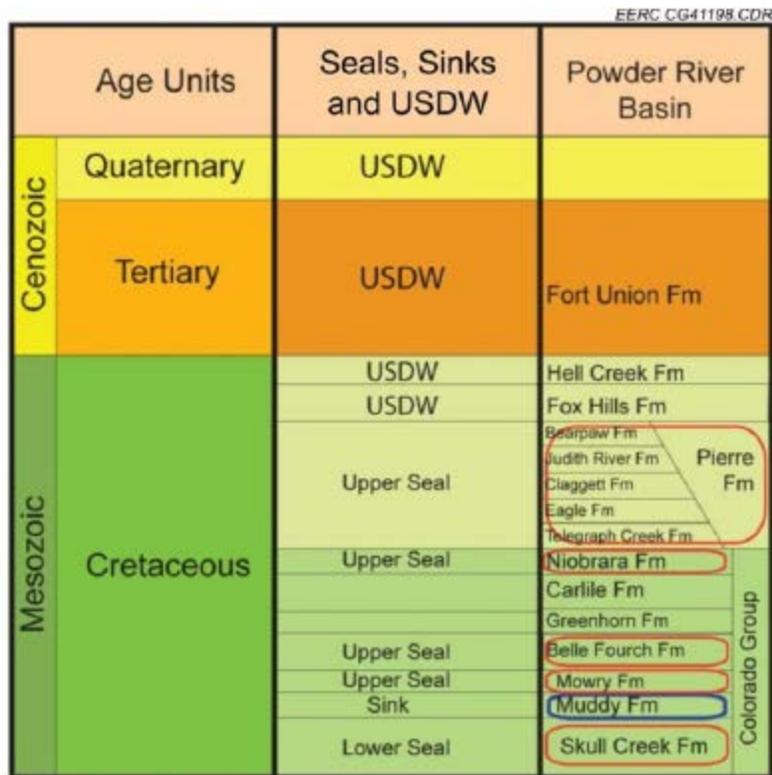
Figure 4-5. Late Cretaceous to Quaternary stratigraphic column of the Powder River Basin. Sealing formations are circled in red, and the injection formation for the Bell Creek demonstration test is circled in blue. Formations bearing USDWs are also identified.
