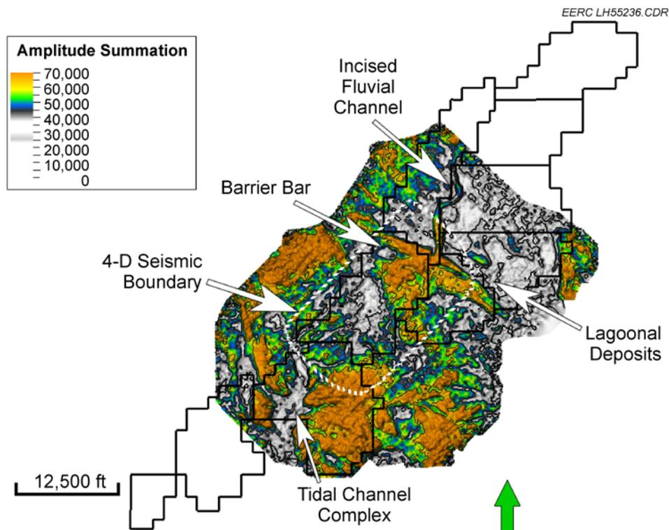
Figure 16. Interpreted amplitude summation map, calculated over the Muddy Formation interval of the Bell Creek Field, with prominent geobodies and a polygon approximating the extent of a 4-D seismic investigation (see Figure 17). Notable in this image is the apparent truncation of the incised fluvial channel near the intersection of the Phase Areas 1, 2, 3, and 4.
