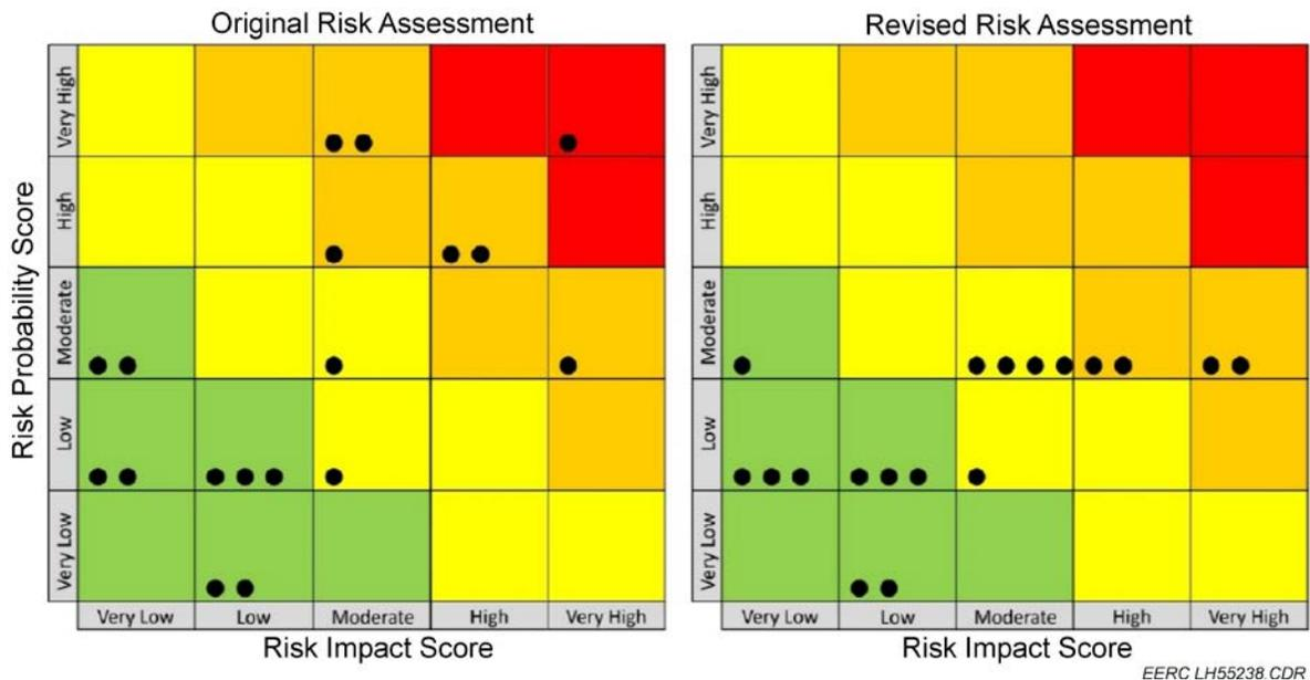
Figure 12. Risk maps showing the assessed values of probability and impact scores for CO<sub>2</sub> containment-related risks associated with an original injection well location (original risk assessment; left panel) and an alternate injection well location (revised risk assessment; right panel) (adapted from Azzolina and others, 2017).
