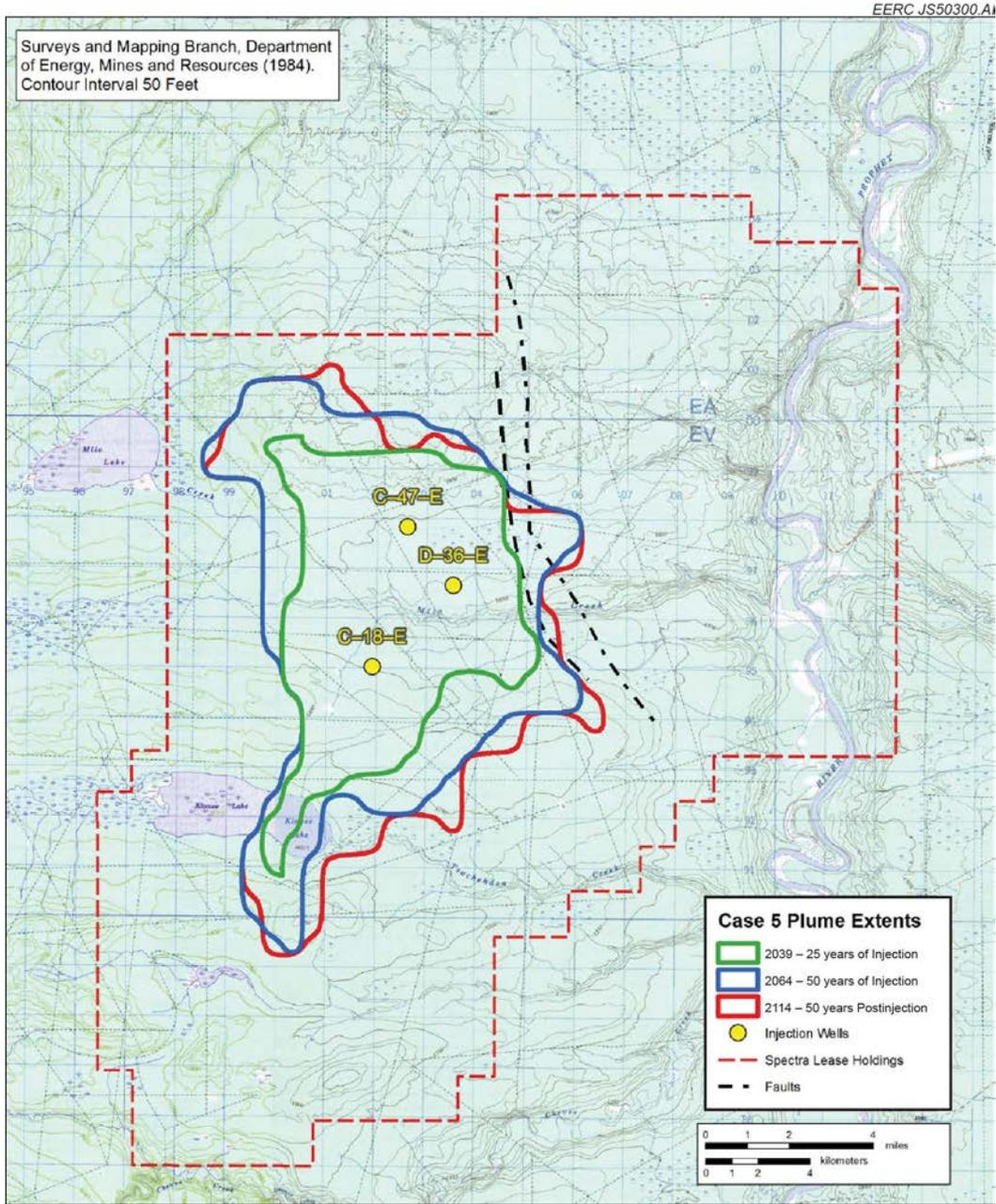
Figure 4-3. Map of predicted plume extents over time for one of the potential injection scenarios at the Fort Nelson site, showing also well locations for monitoring activities.
