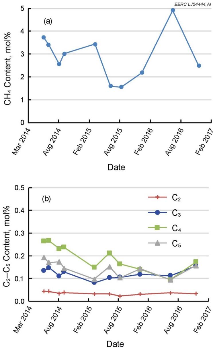
Figure 9-8. Content of hydrocarbons in the produced CO<sub>2</sub> stream: a) for CH<sub>4</sub> and b) for C<sub>2</sub>–C<sub>5</sub>.
