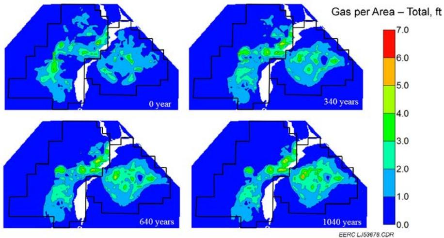
Figure 11-2. Post-WAG injection CO<sub>2</sub> saturation distribution through time in Phase Areas 1 and 2 of the Bell Creek oil field (Peterson and others, 2017).
