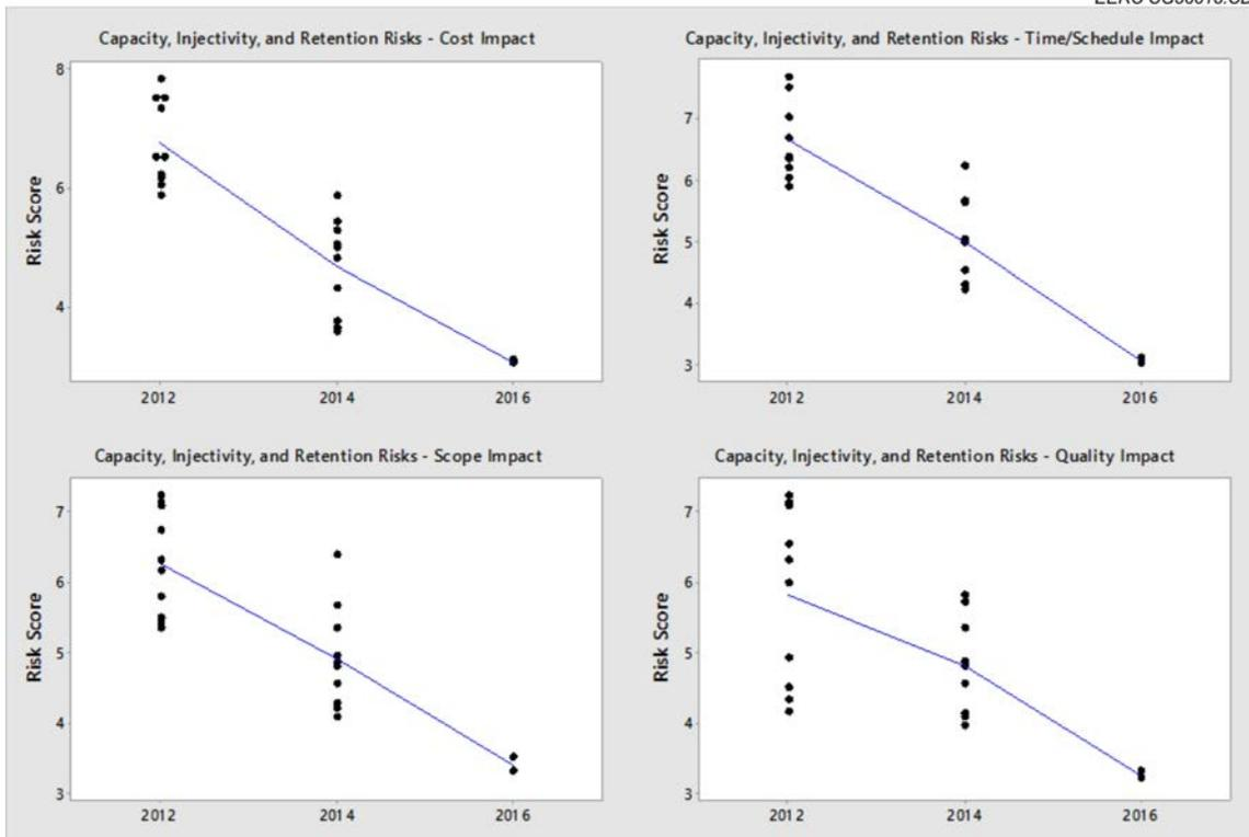
Figure 14. Risk scores evaluated over time (years 2012 to 2016) for Bell Creek risks related to CO<sub>2</sub> storage capacity, injectivity, and retention for impacts to cost (upper left), time/schedule (upper right), scope (lower left), and quality (lower right). A horizontal “jitter” has been added to the *x*-direction for points with similar risk scores (for data points with identical risk scores, they are separated by a small horizontal distance, or jitter, so that they are visible).
