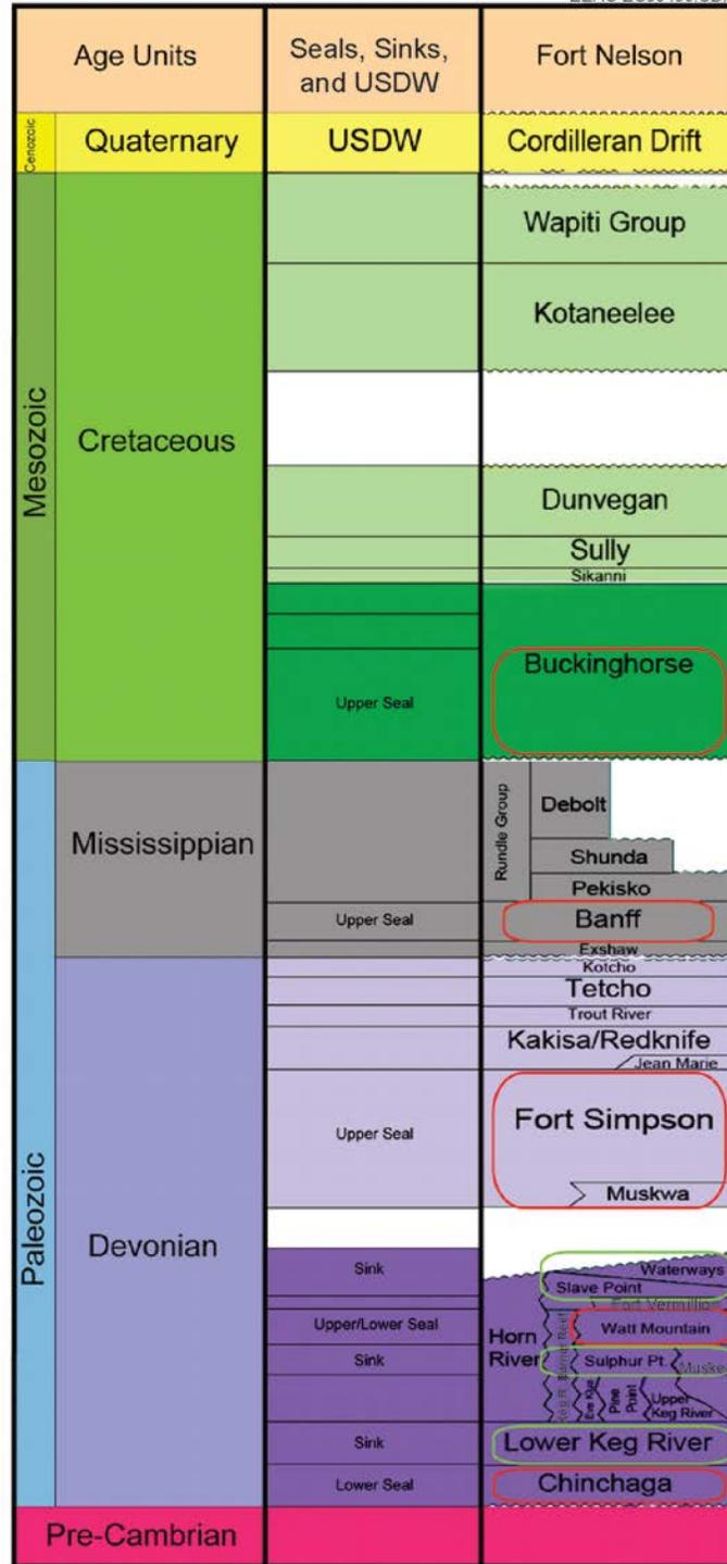
Figure 4-2. Stratigraphic column of the Fort Nelson area (Sorensen and others, 2014). The target injection zones are the Slave Point, Sulphur Point, and Lower Keg River formations. The overlying Fort Simpson and Muskwa shales (~550 m thick) represent an impermeable seal. (USDW is an underground source of drinking water.)
