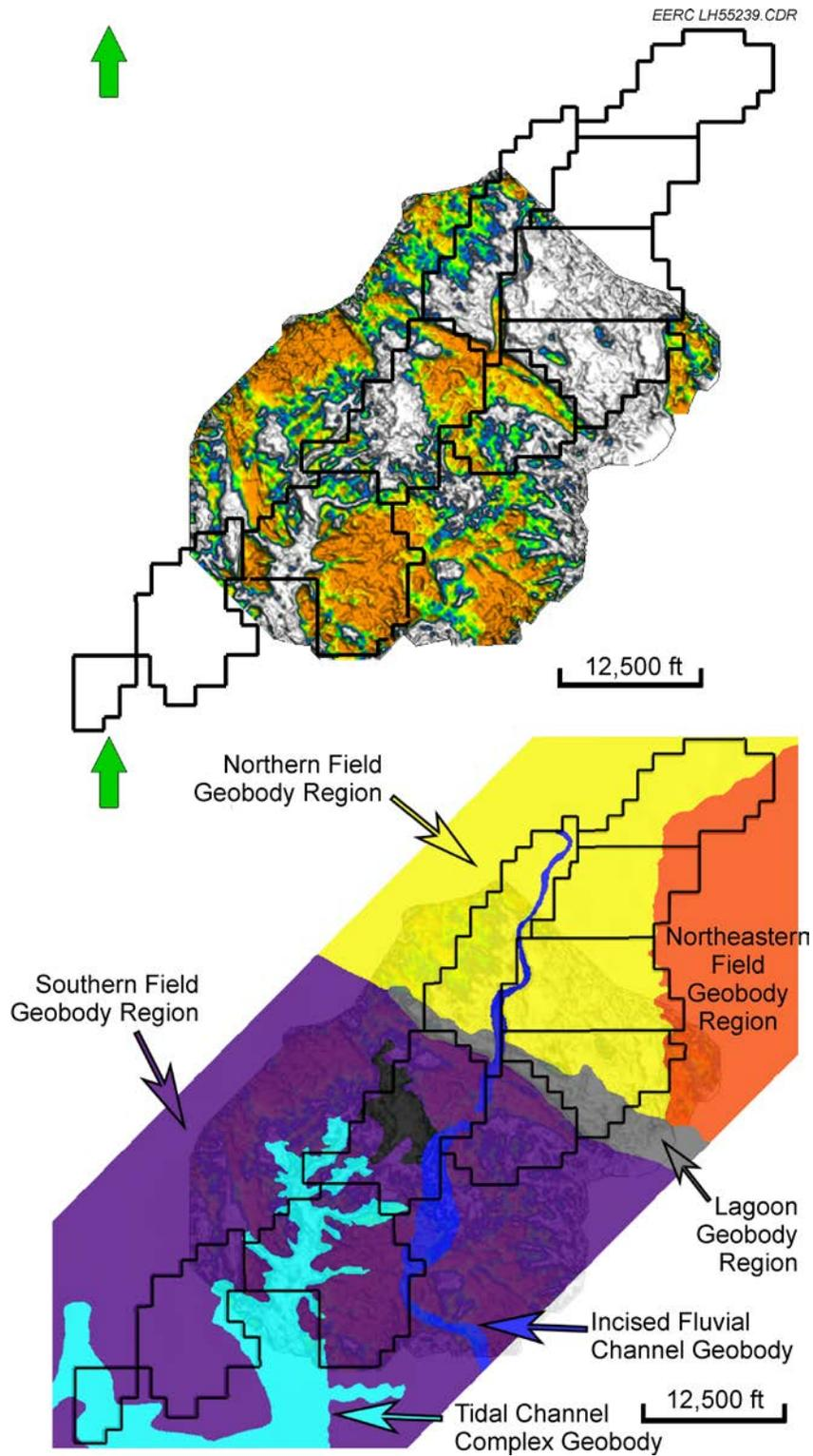
Figure 10. Amplitude summation map calculated over the Muddy Formation interval of the Bell Creek Field (top; adapted from Burnison and others, 2014) and a semitransparent geobody region overlay with the amplitude map (bottom).
