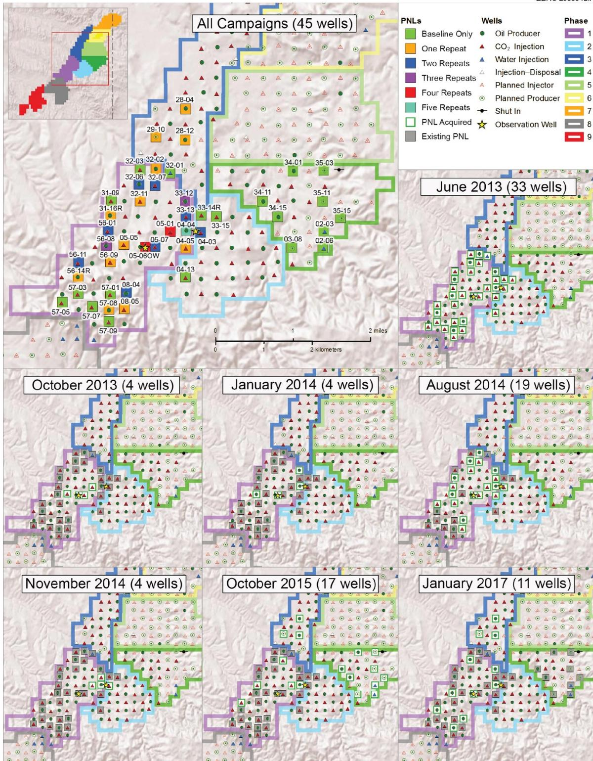
Figure 9-1. Bell Creek Field map showing where baseline and repeat/monitor pass PNLs have been collected since 2013 and also which wells were logged in each campaign (Jin and others, 2017a).
