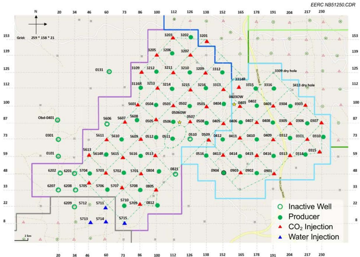
Figure 5-2. Example of the 40-acre five-spot injection/production pattern being implemented at the Bell Creek demonstration test. Injection and producer wells are depicted for Phase Areas 1 (outlined in purple) and 2 (outlined in blue) of the site.
