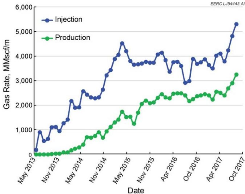
Figure 9-7. CO<sub>2</sub> injection and production rates during the CO<sub>2</sub> EOR process.
