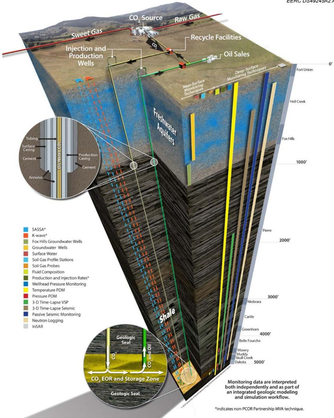
Figure 15. Stratigraphic column of the Bell Creek Field illustrating individual MVA techniques applied as part of the Bell Creek Project (modified from Hamling, 2013).
