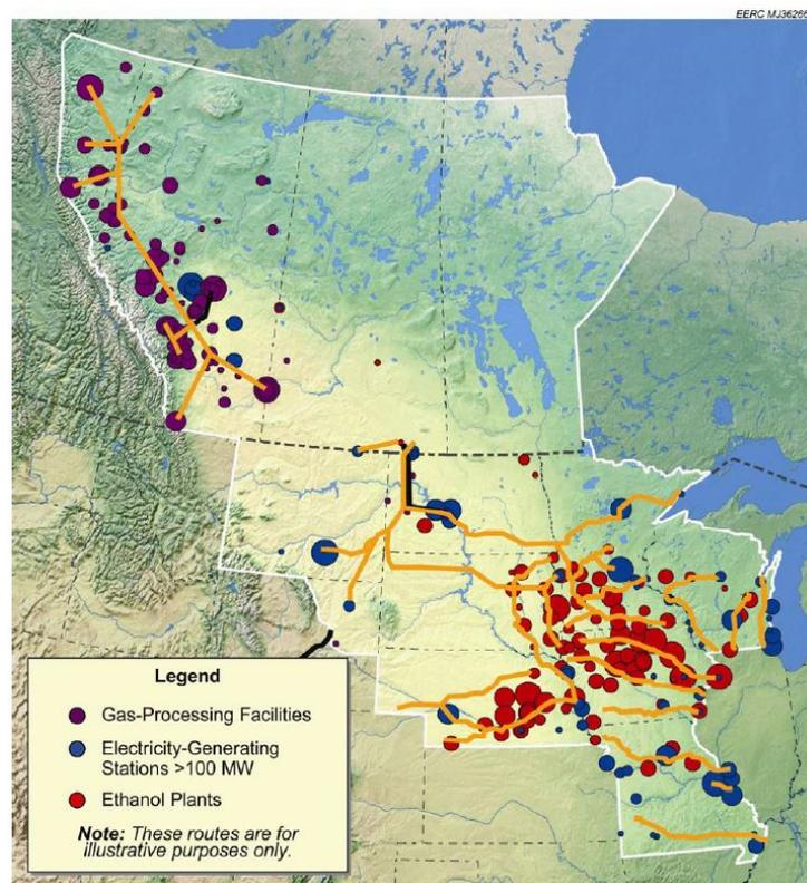
Figure 6-2. Hypothetical CO<sub>2</sub> pipeline network devised for the PCOR Partnership region connecting natural gas-processing, ethanol-producing, and electricity-generating facilities with secure geologic storage sites. Gold lines are hypothetical pipelines; black are existing or planned pipelines.
