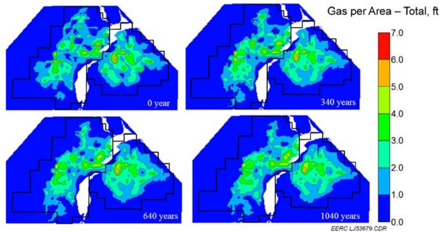
Figure 11-1. Post-CCI CO<sub>2</sub> saturation distribution through time in Phase Areas 1 and 2 of the Bell Creek oil field (Peterson and others, 2017).
