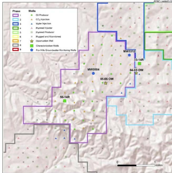
Figure 5-3. Location of monitoring wells drilled within Phase Areas 1 and 2 of the Bell Creek oil field to support PCOR Partnership efforts.
