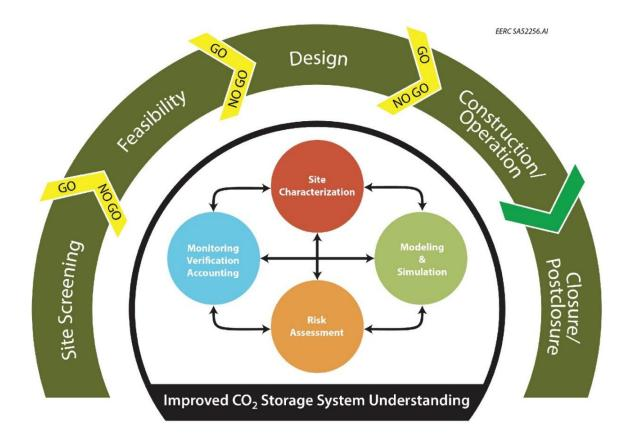
Figure 3. PCOR Partnership AMA for commercial development of CO<sub>2</sub> storage projects (modified from Gorecki and others, 2012). The AMA consists of four primary technical elements (i.e., site characterization, modeling and simulation, risk assessment, and MVA) which are performed at each of the phases of a commercial CO<sub>2</sub> storage project (i.e., site screening, feasibility, design, construction/operation, and closure/postclosure).
