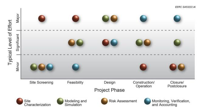
Figure 4. Estimated relative proportion of AMA technical elements performed during each of the project phases of a commercial CO<sub>2</sub> storage project.
