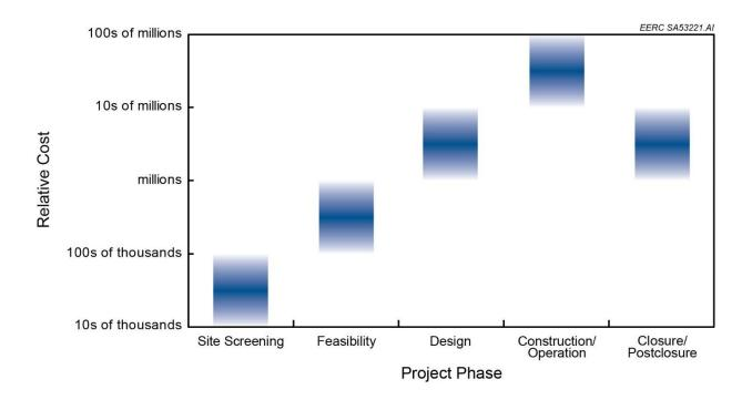
Figure 5. Potential range of approximate total cost for each phase of a CO<sub>2</sub> storage project.
