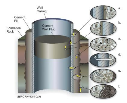
Figure 6. Conceptual illustration of the potential leakage pathways for CO<sub>2</sub> through a well along the casing–cement interface (a and b), within the cement (c), through the casing (d), through fractures (e), and along the cement–formation interface (f) (from Celia and others, 2004).
