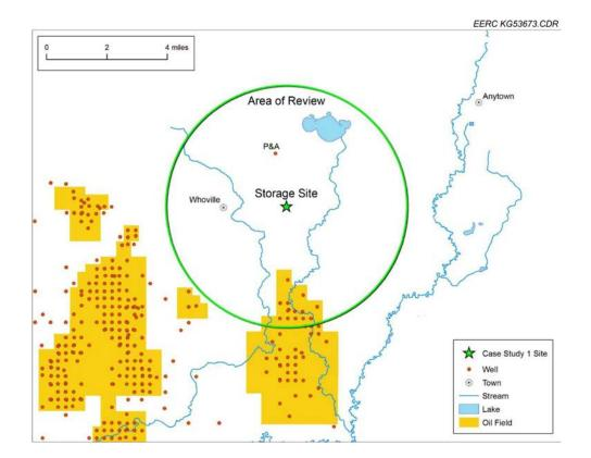
Figure 11. Conceptual map of Case Study 1 showing the planned injection location and estimated AOR based on pressure considerations.
