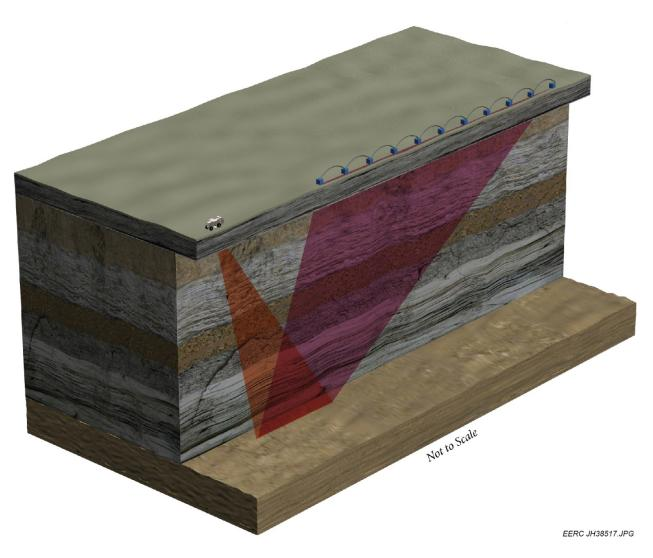
Figure 7. Schematic of 2-D seismic line collection (Hamling and others, 2011).
