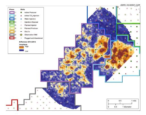
Figure 9. Example 4-D seismic analysis. Areas with greater yellow-to-brown shading indicate regions of greater CO<sub>2</sub> (modified from Salako and others, 2017).
